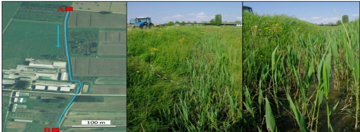
Figure 11: Vegetated ditches for the mitigation of pesticides runoff (Adopted from; Otto et al. 2015)
